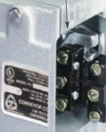
STANDARD SWITCH - One SP/DT switch per end (two switches per end available) • 20 AMPS, 125, 250 or 480 VAC • 10 AMPS, 125 VAC "L" (tungsten lamp load) • 1 HP, 125 VAC • 2 HP, 250 VAC • 1/2 AMP, 125 VDC • 1/4 amp, 250 VDC
